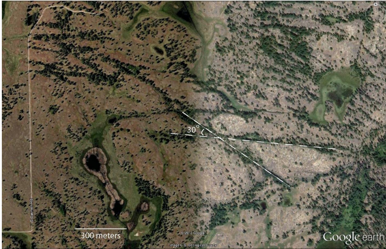
Figure 9. Example of conjugate fractures in the western portion of the Cheney Fracture Zone. The angle between fractures is approximately 30^\circ , with a fracture trending N57^\circ W ( 303^\circ ) and 0.48 miles (775 m) long and a second N85^\circ W ( 275^\circ ) and 0.59 miles (950 m) long.
