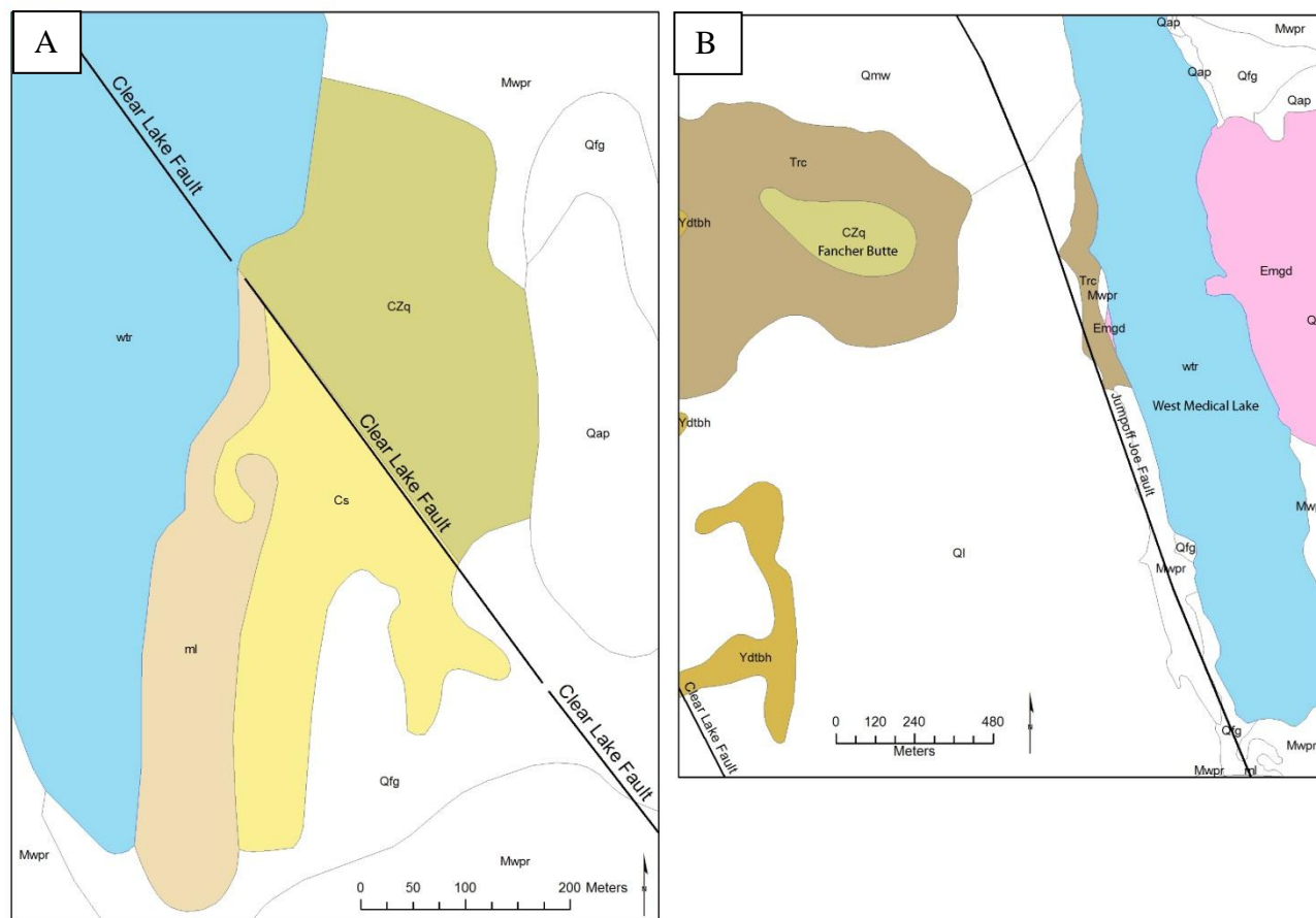
Figure 7. Maps depicting two faults in the West Plains region. A) the normal fault movement along the Clear Lake fault that has uplifted Cambrian quartzite (CZq) relative to the hanging wall, locally composed of Cambrian shale and phyllite (Cs). B) Map illustrating the easternmost outcrop of the Mesoproterozoic Buffalo Hump formation of the Deer Trail Group (Ydtbh) to the west and Eocene granodiorite of Medical Lake (Emgd) to the east. The structural contact is regionally considered the Jumpoff Joe Fault, and is inferred along the west side of West Medical Lake based up on mapping by Joseph (1990).
