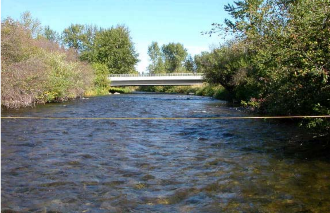
PHOTOGRAPH 16. LSR @ PINE RIVER PARK – UPSTREAM VIEW. 9/25/2002, 12:00. Measured Flow: 106.1 cfs. Flow at Dartford: 117 cfs. Weather: Sunny. Streamflow Conditions: Stable.
