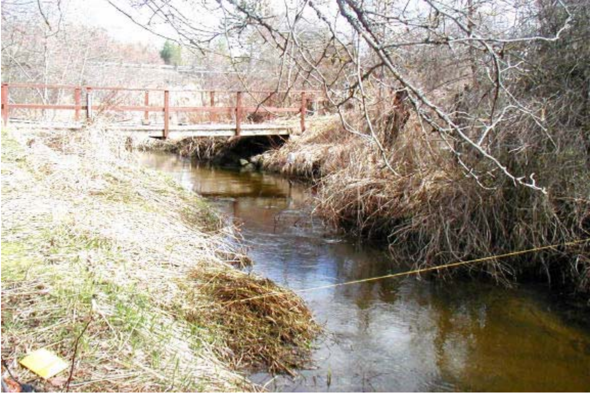
PHOTOGRAPH 58. OTTER CREEK – UPSTREAM VIEW. 3/27/2003, 12:00. Measured Flow: 10.1 cfs. Flow at Dartford: 894 cfs. Weather: Overcast. Streamflow Conditions: Stable.
