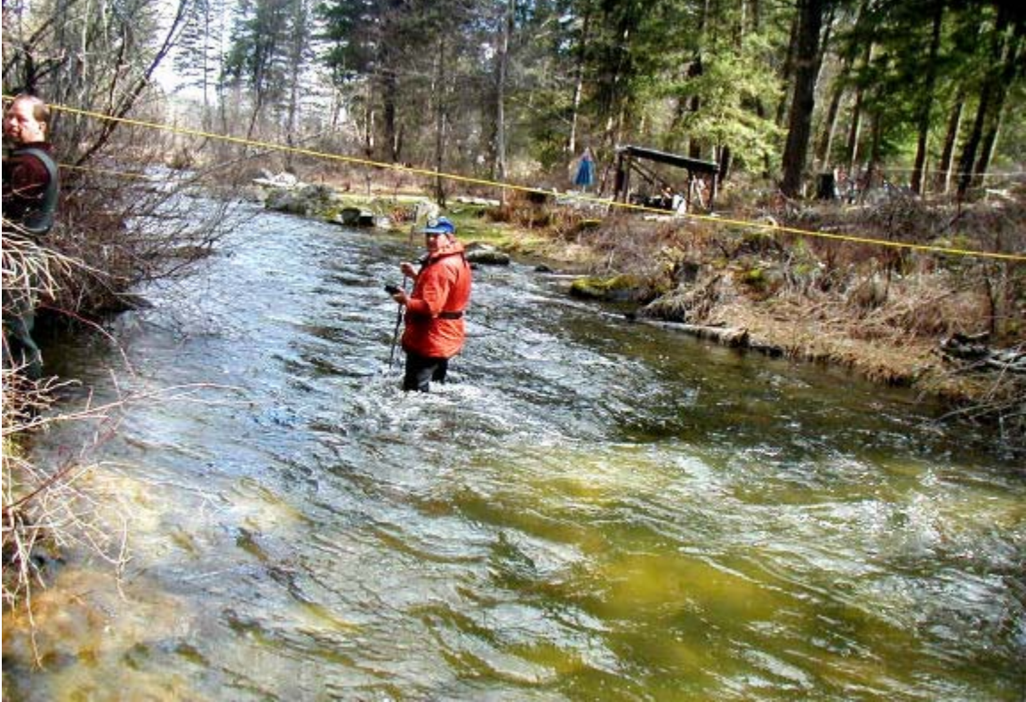
PHOTOGRAPH 30. LSR @ ELK PARK – UPSTREAM VIEW. 3/27/2003, 10:00. Measured Flow: 69.3 cfs. Flow at Dartford: 894 cfs. Weather: Overcast. Streamflow Conditions: Stable.
