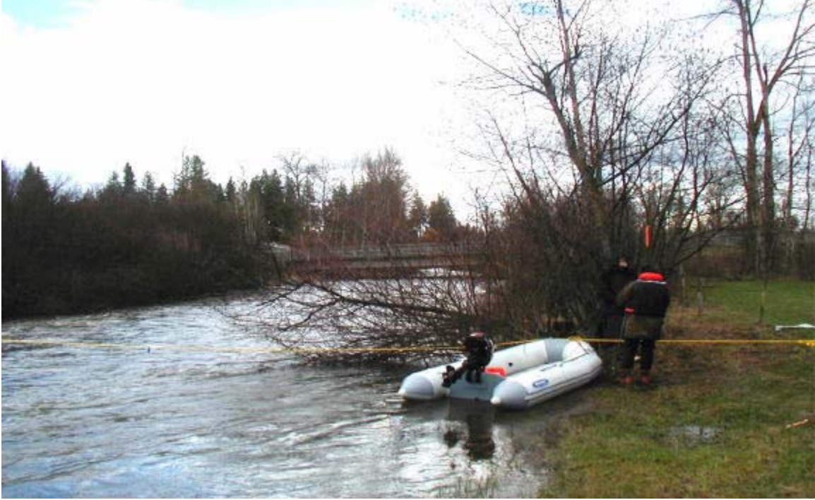
PHOTOGRAPH 20. LSR @ PINE RIVER PARK – UPSTREAM VIEW. 3/26/2003, 13:00. Measured Flow: 868.1 cfs. Flow at Dartford: 828 cfs. Weather: Overcast. Streamflow Conditions: Somewhat Variable.
